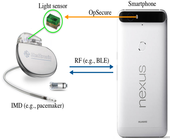
Fig. 2. The IMD (pacemaker) has an embedded light sensor, and the smartphone flashlight acts as a light source.
