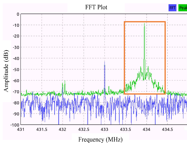
Fig. 3. The door sensor generates a packet as soon as it detects the door is open. The spike in the fast Fourier transform of the analog signal shows a single transmission using OOK modulation.
