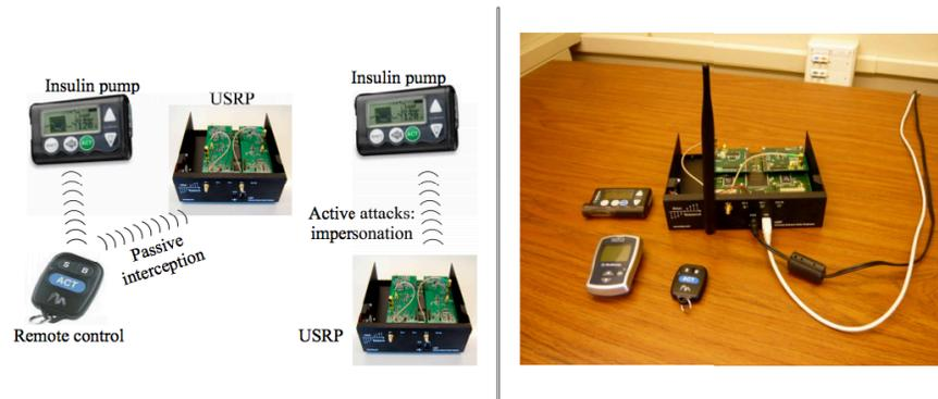
**Figure 5.3:** Security attacks and the experimental setup [Li et al., 2011].
